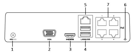
\*: The rear panel of NVR-108H-D/8P provides 8 PoE interfaces.
