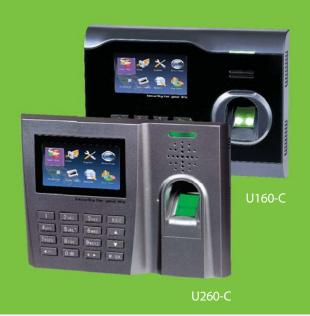
U160-C / U260-C is a biometric fingerprint Time & Attendance terminal with 3"TFT display. Easy to install, and with a modern design, it is the perfect solution for small installations. It incorporates the ZK fingerprint Sensor. The color TFT display offer users easy menu management. It can connect to Time & Attendance management software by Ethernet or USB port, and also operate on standalone mode, downloading data by USB pendrive. Optionally, it can incorporate a proximity reader.
