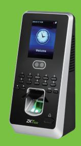
MultiBio 800-H is a time attendance and access control terminal for face and fingerprint verification. Using ZK lastest ZKFACE 7.0 high-speed face recognition algorithm, it has extremely high verification speed and low error rate.
